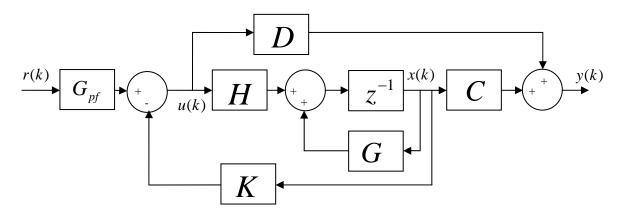
Here  $G_{pf}$  is the <u>prefilter gain</u>, r(k) is the <u>reference input</u>, and  $K = \begin{bmatrix} k_1 & k_2 \end{bmatrix}$  is the <u>feedback gain</u> matrix. The state variable model for the plant is assumed to be
