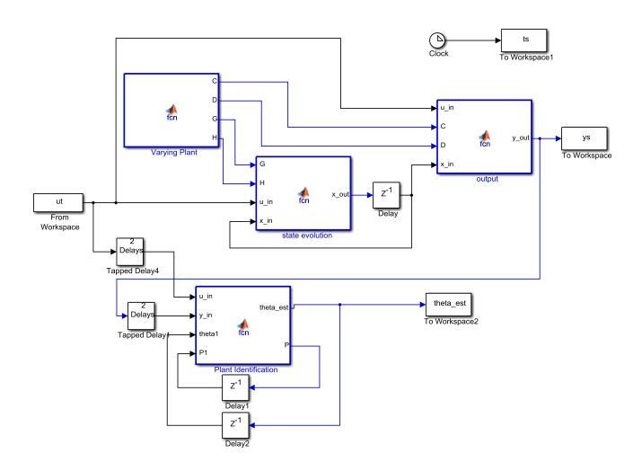
You need to run **plant\_identification\_driver.m** and show that the Matlab and Simulink results for the plant are the same. You will need some code like the following in your plant identification block to initialize the algorithms
