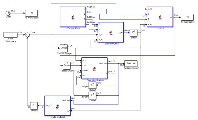
Note that your state feedback block now needs to use the computed parameter estimates to determine the correct feedback gains. You will need to include code like the following to go from the transfer function coefficient estimates to a state variable model in controllable canonical form:
