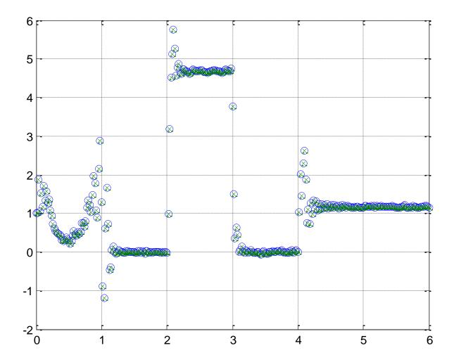
At this point you should be elated that you got all of this to work, and disappointed that this is a pretty poor control system—the output is not following the input. This can be fixed by including an integrator in our system or adaptively changing the prefilter gain, which is easier and we will do that next.
