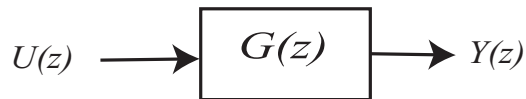
Figure 5: Discrete-time transfer function, G(z) = \frac{Y(z)}{U(z)} . Discrete-time transfer functions are often implemented in terms of the difference equation they represent.
