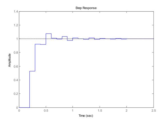
Figure 1. Discrete-time example with w PI controller.
