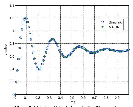
Figure 7. Matlab and Simulink results for PD controller.
