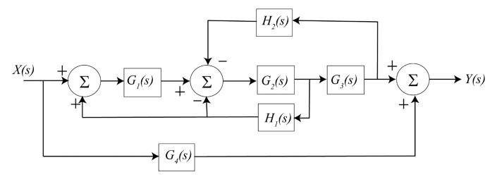
Problems 6 - 8 refer to the signal flow graph representation of the following block diagram.
