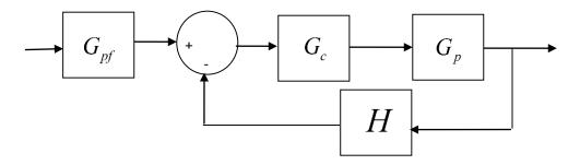
31) To reduce the sensitivity of the closed loop transfer function variations in the plant G<sub>p</sub>, we should
