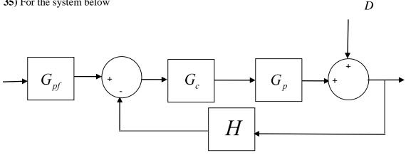
to reduce the effects of the external disturbance D on the system output, we should a) make  $|G_c(j\omega)G_p(j\omega)H(j\omega)|$  large b) make  $|G_c(j\omega)G_p(j\omega)H(j\omega)|$  small
