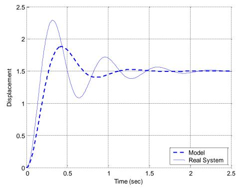
13) In order to make the model better match the real system, the *damping ratio* of the *model* should bea) increased b) decreased c) left alone d) impossible to determine
