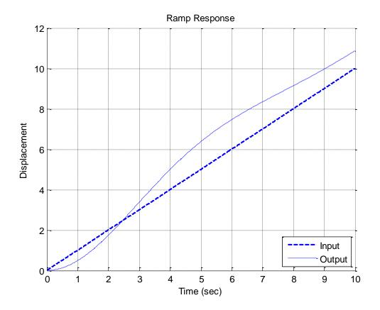
The best estimate of the **steady state error** is a) 0.75 b) -0.75 c) 1.5 d) -0.5 Problems 11 and 12 refer to a system with poles at -2+5j. -2-5j. -10+j, -10-j, and -20
