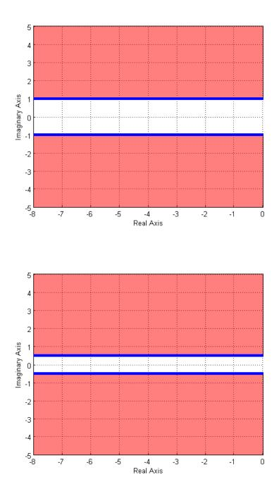
**25**) One of the shaded regions below shows the possible pole locations for a percent overshoot less than 10%, and the other shows the possible pole locations for a percent overshoot less than 20%. Which of the two graphs shows the possible pole locations for a percent overshoot less than 20%?
