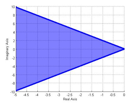
**22)** The (dark) shaded area in the s-plane figure below shows the possible pole location for an ideal second order system that meets which of the following constraints?
