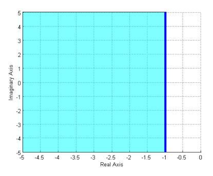
**20)** The (dark) shaded area in the s-plane figure below shows the possible pole location for an ideal second order system that meets which of the following constraints?
