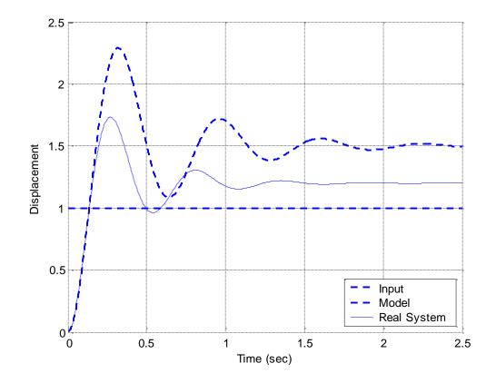
16) In order to make the model better match the real system, the <u>damping ratio</u> of the *model* should bea) increased b) decreased c) left alone d) impossible to determine
