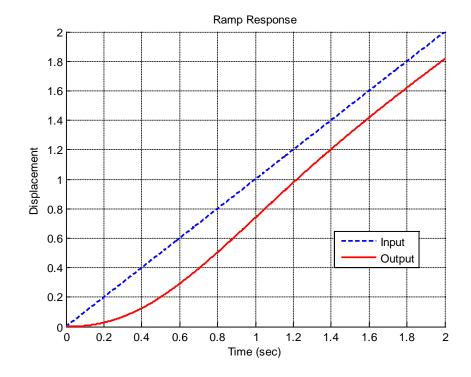
7) Estimate the steady state error for the ramp response of the system shown below:
