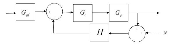
to reduce the effects of sensor noise N on the closed loop system, we should a) make  $|G_c(j\omega)G_p(j\omega)H(j\omega)|$  large b) make  $|G_c(j\omega)G_p(j\omega)H(j\omega)|$  small c) make  $|H(j\omega)|$  large d) do nothing, we cannot change the sensitivity
