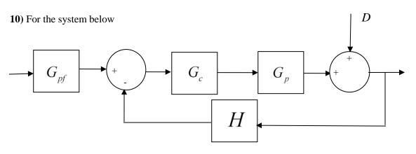
to reduce the effects of the external disturbance D on the system output, we should
