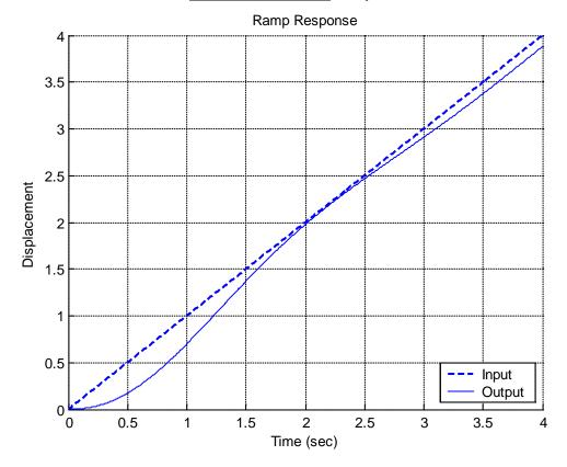
Problems 11 and 12 refer to the **unit ramp response** of a system, shown below:
