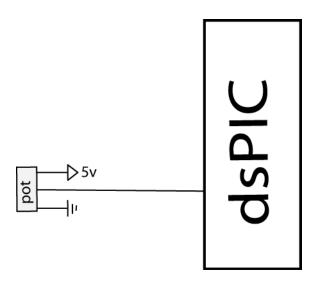
Part J (Changing the dutycycle value by reading from the potentiometer)
