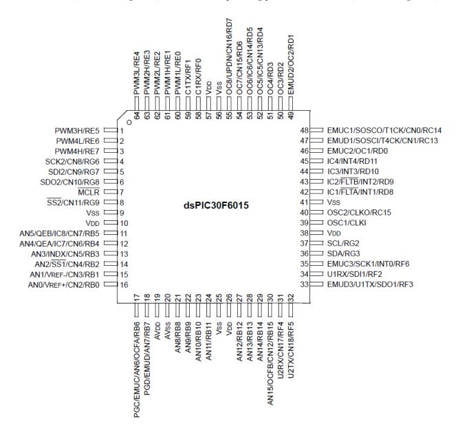
Figure 1. dsPIC30F6015 64-PIN pinout.
