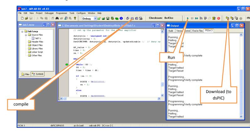
You should **compile** the existing program, **download** it to the dsPIC, and **run** it. You should see a sequence of numbers on your screen (the secure CRT screen). These correspond to sample times.
