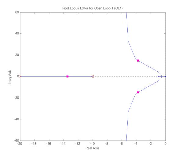
**10)** Based on this root locus plot, the best estimate of the poles of the closed loop system are
