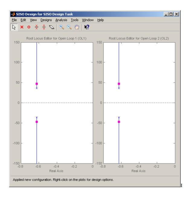
Let's initially assume we want to use a PI-D controller. In this case, for simulation purposes, we have  $C_2(s) = k_d s$  (we won't worry about the lowpass filter here). We will start off assuming  $k_d = 0.01$ , but this is just a guess! To assign this to controller C2, in the design window we select **Designs**, the **Edit Compensator**, then select **C2** in the compensator window, and enter the controller.
