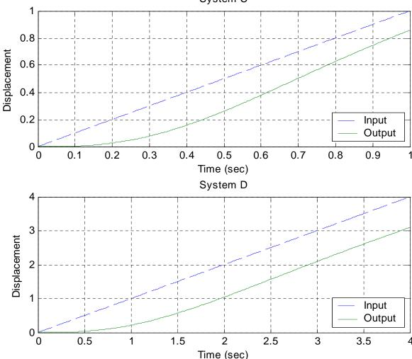
Figure 2. Ramp responses for systems C and D.
