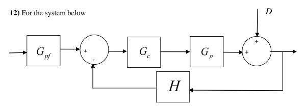
to reduce the effects of the external disturbance D on the system output, we should a) make  $|G_c(j\omega)G_p(j\omega)H(j\omega)|$  large b) make  $|G_c(j\omega)G_p(j\omega)H(j\omega)|$  small c) make  $G_{pf}$  large d) do nothing, we cannot change the sensitivity
