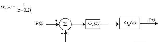
*Hint:* Drawing a root locus plot for a discrete-time system is identical to drawing the root locus plot for a continuous time system (treat z as you would s). The only difference is the interpretation.
