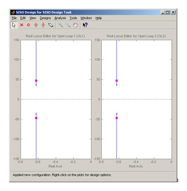
Let's initially assume we want to use a PI-D controller. In this case, for simulation purposes, we have  $C_2(s) = k_d s$  (we won't worry about the lowpass filter here). We will start off asuming  $k_d = 0.01$ , but this is just a guess! To assign this to controller C2, in the design window we select **Designs**, the **Edit Compensator**, then select **C2** in the compensator window, and enter the controller.
