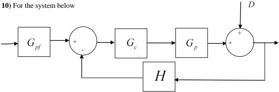
to reduce the effects of the external disturbance D on the system output, we should
