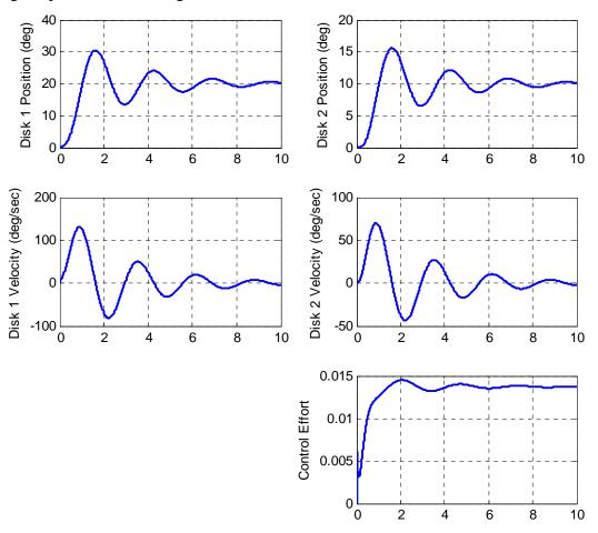
**Figure 6.** Integral control of a 2 dof system with bad data. We are controlling the position of the second disk (problem 2d).
