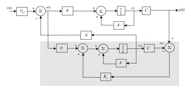
Figure 8. Full order observer state variable feedback structure.
