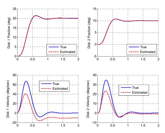
**Figure 23.** State feedback, full order observer, and integral control for the 2 dof system with a bad model (problem 6d).
