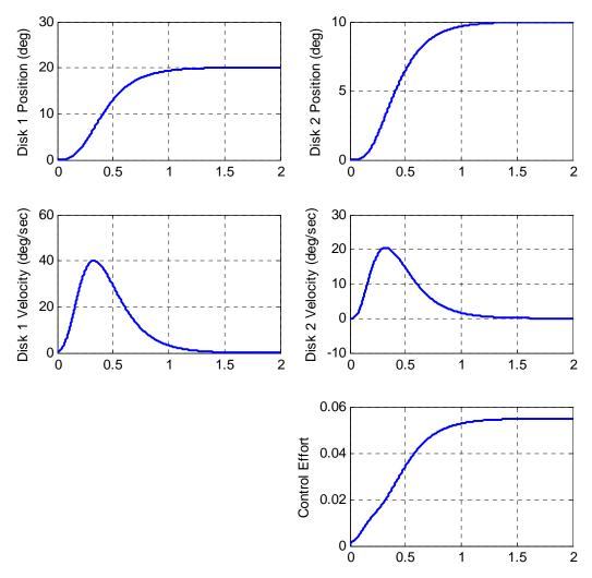
**Figure 5.** Integral control of a two degree of freedom system. We care controlling the position of the second disk (part 2c).
