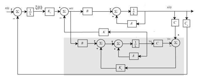
**Figure 17.** Full order observer state variable feedback structure with integral control.
