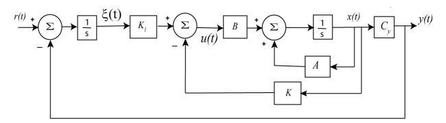
Figure 1. Integral control structure.
