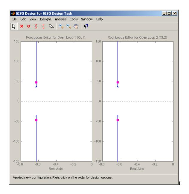
Let's initially assume we want to use a PI-D controller. In this case, for simulation purposes, we have  $C_2(s) = k_d s$  (we won't worry about the lowpass filter here). We will start off asuming  $k_d = 0.01$ , but this is just a guess! To assign this to controller C2, in the design window we select **Designs**, the **Edit Compensator**, then select **C2** in the compensator window, and enter the controller.
