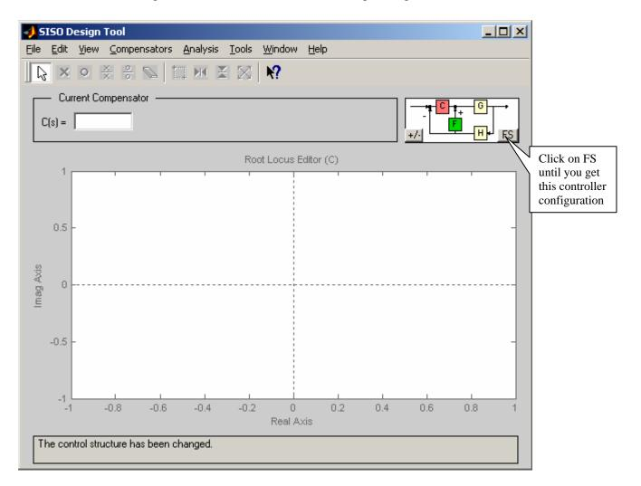
Sisotool will allow us to modify both C(s) and F(s), but it is much easier to modify C(s). We will have to iterate between both of these.
