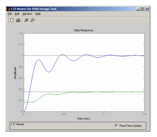
The step response for this controller configuration is:
