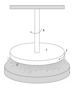
By drawing a free body diagram and balancing torques, we get the equation of motion
