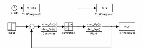
This is a <u>closed loop</u> system, in that we are feeding back the output and comparing this output to what we wanted the output to be. We have also added a new transfer function, the *controller* or *compensator*, usually denoted as Gc(s).
