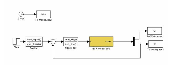
This is a cross between **closedloop.mdl** and **Model205\_Openloop.mdl.**, so you can pretty much just cut and paste. Note that if you want to scale to degrees, you must do this after the feedback branch.
