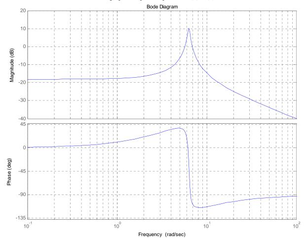
23) The gain crossover frequency used to determine the phase margin for this system is best estimated as
