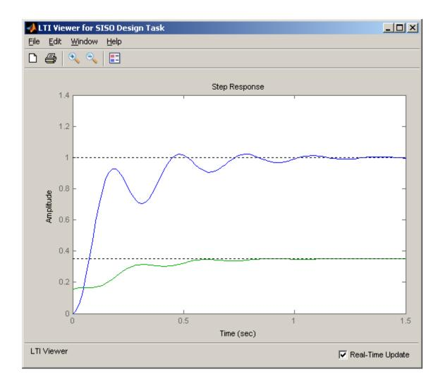
Note that, compared to a normal PID controller, the control effort is not infinite at 0, and actually builds as time goes on (like an integral controller). At this point we might want to go back modify our controllers C1 and C2 to see if we get acceptable performance. Note that we can modify the two controllers (and gains) independently.
