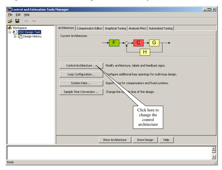
Next we need to select the correct architecture. Select the following architecture and be sure that sisotool uses negative feedback for both loops.
