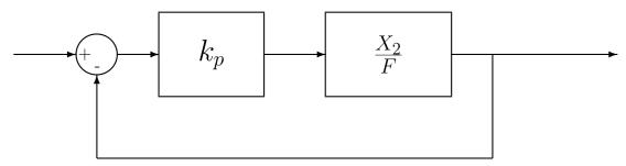
For a step response of amplitude Amp, show that the steady state value of  $x_2(t)$ ,  $x_{2,ss}$  is
