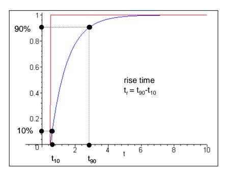
Figure 3. Step response of the RC lowpass filter circuit of Figure 1, showing the definition of the 10-90% risetime.
