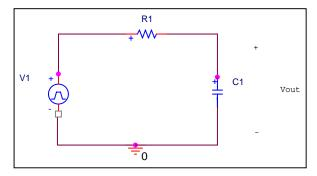
Figure 2. Simple RC lowpass filter circuit.
