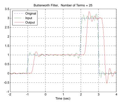
Figure 1. Input and Fourier series representation of the input and output using a 10<sup>th</sup> order Butterworth filter.
