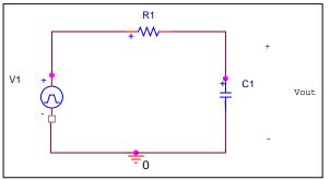
Figure 1. Simple RC lowpass filter circuit.
