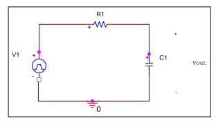
Figure 2. Simple RC lowpass filter circuit.
