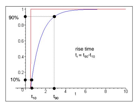
Figure 2. Step response of the RC lowpass filter circuit of Figure 1, showing the definition of the 10-90% risetime.
