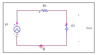
Figure 1. Simple RC lowpass filter circuit.
