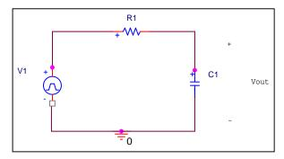
Figure 1. Simple RC lowpass filter circuit.
