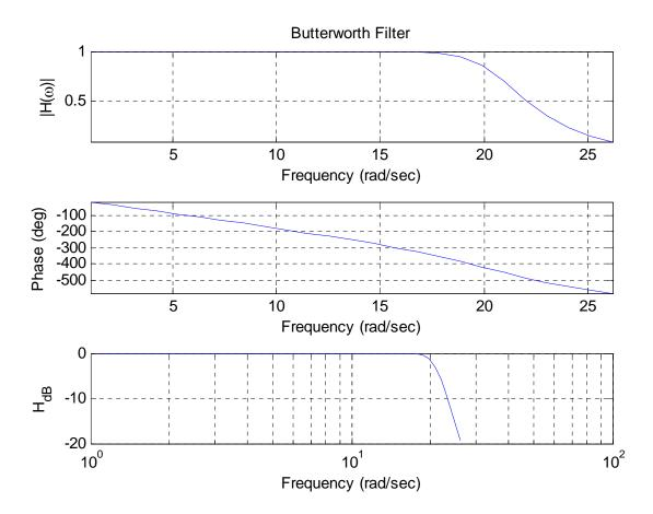
Figure 2. Frequency response of the 10<sup>th</sup> order Butterworth filter.
