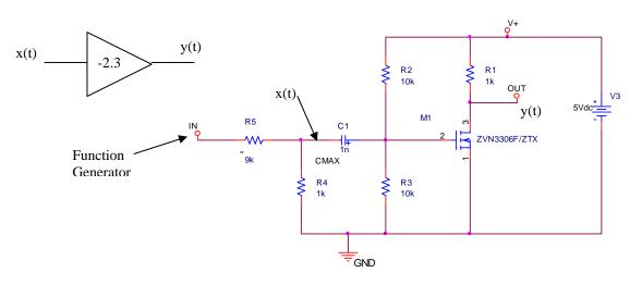
Figure 1: Circuit Diagram of the common-source amplifier. The ideal block diagram representation for this amplifier is shown as the triangle in the upper left.
