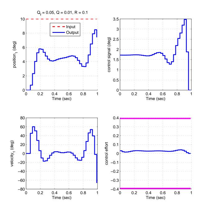
Figure 1: Initial results from the one degree of freedom torsional system using Q = 0.01, R = 0.1 and  $Q_f = 0.05$
