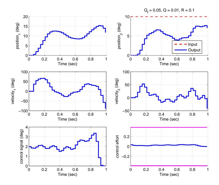
Figure 2: Initial results from the two degree of freedom torsional system controlling the position of the second disk using Q = 0.01, R = 0.1 and  $Q_f = 0.05$
