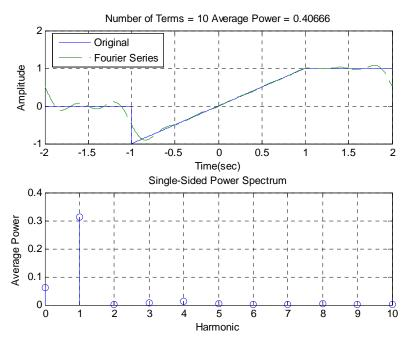
Figure 5: The single-sided power spectrum of f(t).
