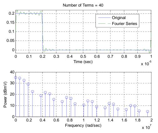
Figure 2: Plot for 8c-(i), Amplitude = 0.2V,  $\tau = 2\mu s$ , and  $T = 10\mu s$ .
