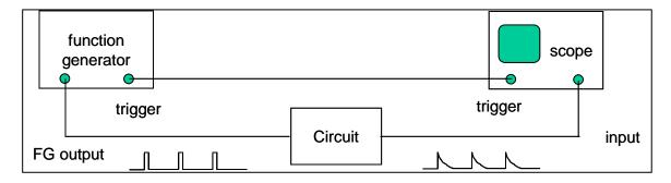
Figure 4. Experimental test setup for measuring the impulse and step response of the SUT.
