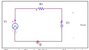
Figure 1. Simple RC lowpass filter circuit.
