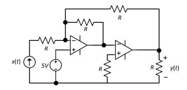
Careful: Be sure to account for the 5V voltage source at the positive terminal of the first op-amp.
