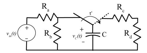
Assume the system is initially at rest (initial conditions are zero), the input is a step of amplitude 4V, and the static gain is 0.5. Also assume the time constant during charging the capacitor is 1 ms, and the time constant during discharging the capacitor is 2 ms. The switch is connected to the source (charging the capacitor) until time  $t^* = 10 \, ms$  The following table may be helpful
