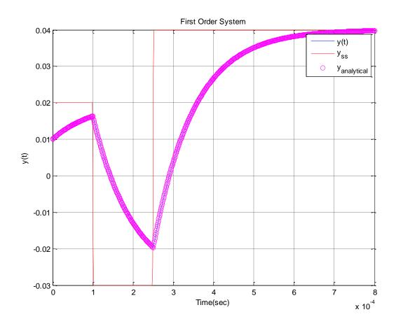
In this figure, it is difficult to really see the difference between the analytical and Simulink solutions. This is because we are using so many data points. One of the ways to get around this is to downsample the time. Let's define a new variable (before the print command and after we have run the simulation)
