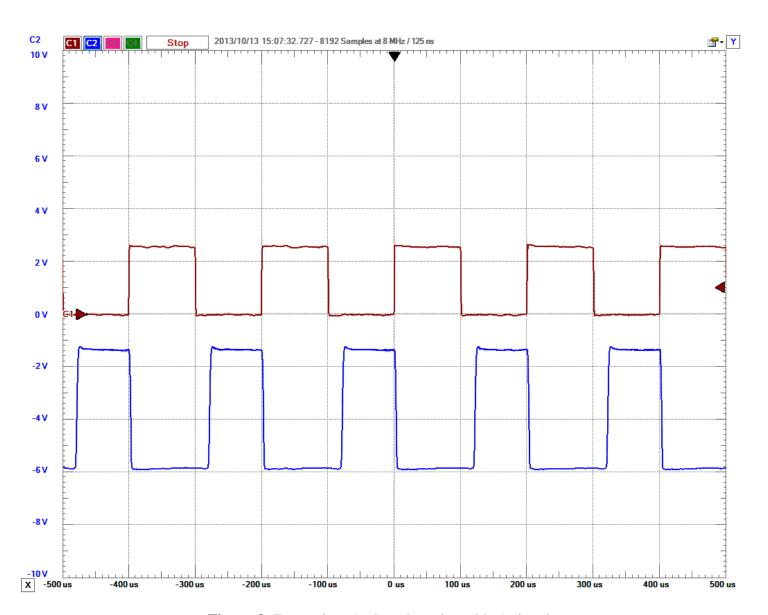
Figure 8. Transmitter (red) and receiver (blue) signal.
