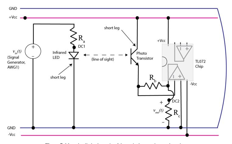
**Figure 7.** More detailed schematic of the optical transmitter and receiver.
