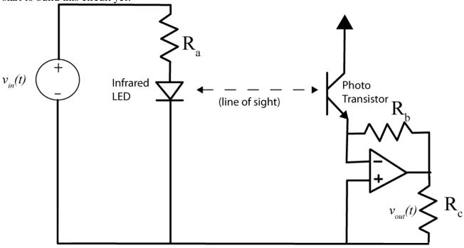
Figure 4. General schematic of optical transmitter and receiver.
