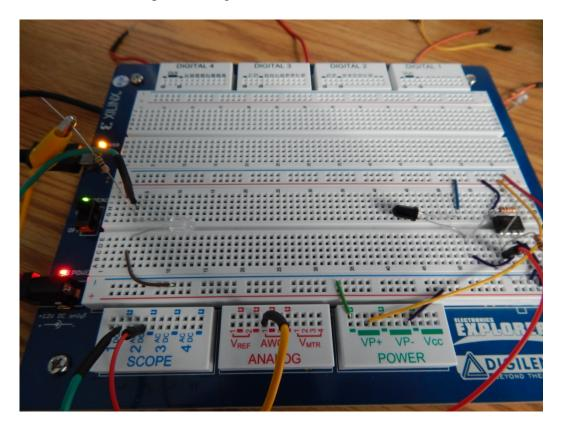
Figure 6. Final circuit with the transmitter and receiver separated.
