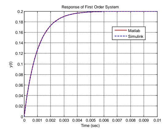
**Figure 1.** Response of first order system to a step of amplitude 0.1
