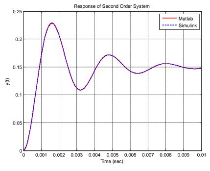
**Figure 3.** Response of second order system to a step of amplitude 0.1
