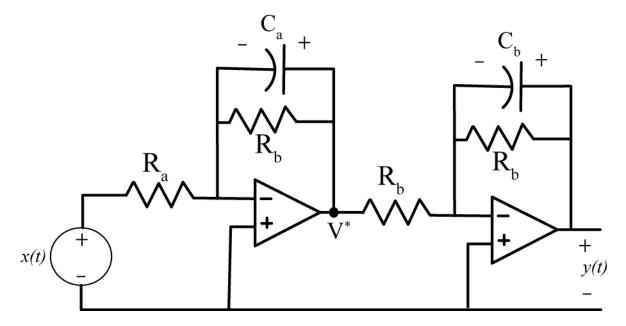
Hint: Write the equations for each op amp in terms of  $V^*$ , and then eliminate this node voltage.
