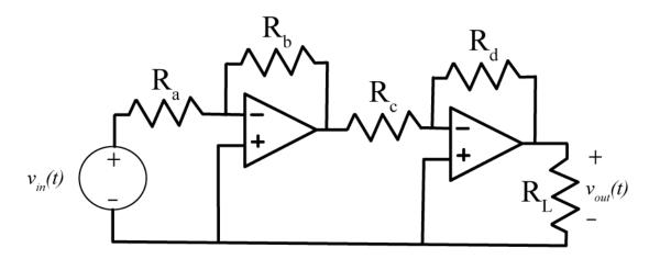
7) For the following circuit, show that  $v_{out}(t) = \left(-\frac{R_e}{R_d} \frac{R_b}{R_a + R_b}\right) v_{in}(t)$
