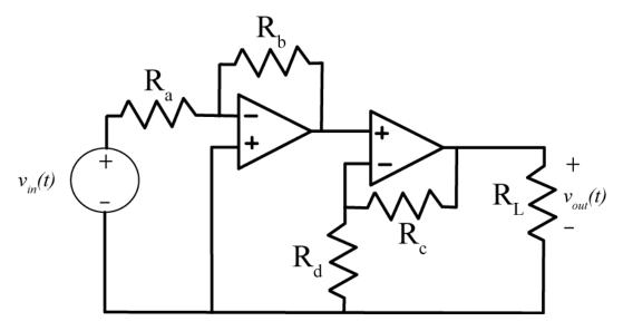
Note that the polarity of the two op-amps are different!
