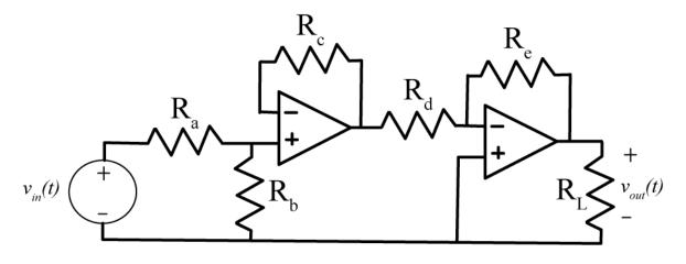
**8)** For the following circuit, show that  $v_{out}(t) = \left(-\frac{R_b}{R_a} \frac{R_c + R_d}{R_d}\right) v_{in}(t)$
