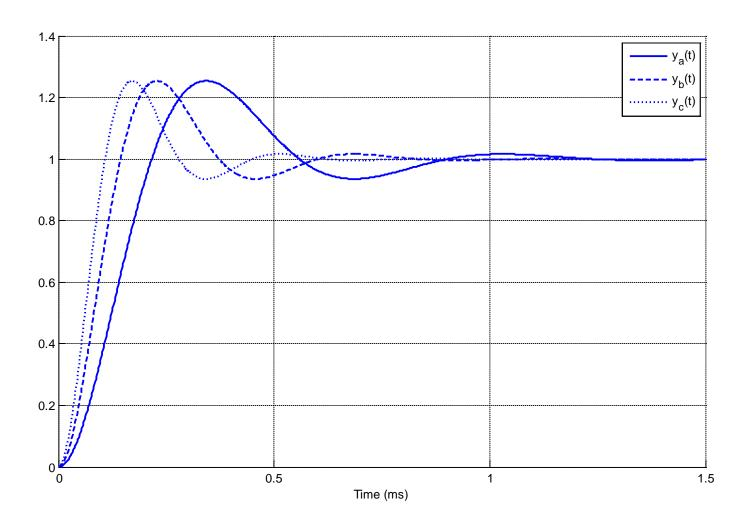
Problems 15-18 refer the following graph showing the response of a second order system to a step input.
