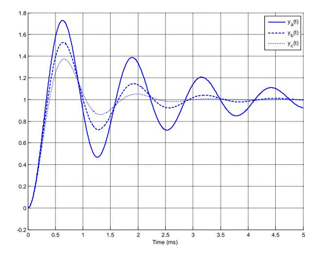
14) The following figure shows the step response of three systems. The only difference between the systems is the natural frequency,  $\omega_n$ .
