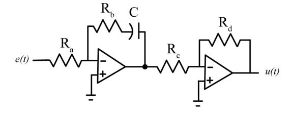
**b)** The following circuit can be used to implement the PD controller  $G_c(s) = \frac{U(s)}{E(s)} = k_p + k_d s$ Determine expressions for  $k_p$  and  $k_d$  in terms of the parameters given in the circuit.
