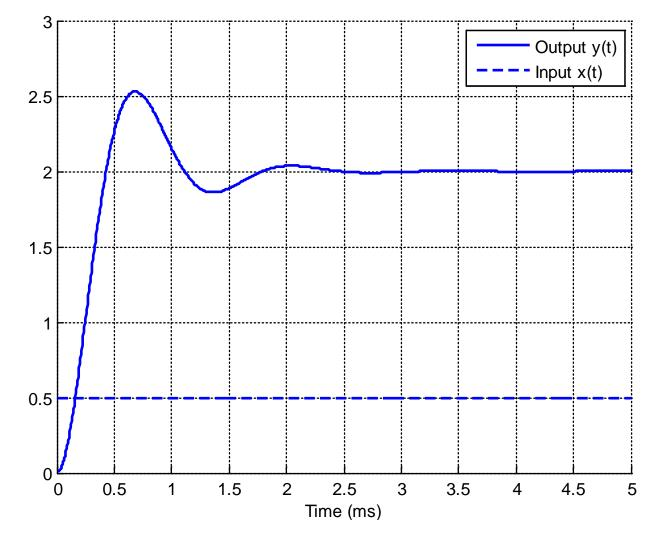
Problems 8-10 refer the following graph showing the response of a second order system to a step input.
