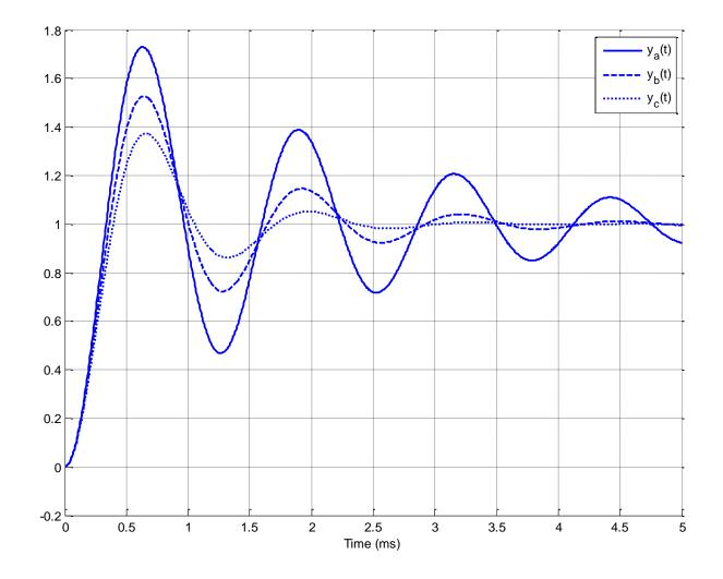
14) The following figure shows the step response of three systems. The only difference between the systems is the natural frequency,  $\omega_{\scriptscriptstyle n}$ .
