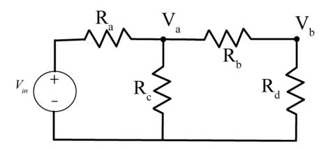
**b**) Create m-files to set up and solve matrix equations for the node values for the following circuit. Use <u>both</u> methods from the Appendix to set up the system of equations.
