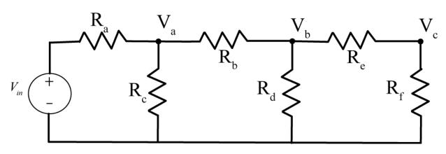
**c**) Create m-files to set up and solve matrix equations for the node values for the following circuit. Use <u>both</u> methods from the Appendix to set up the system of equations.
